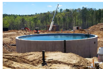
Each structure of the WTP designed to hold water had to be leak tested before it was accepted. Here, the thickener tank was filled for leak testing. The tank was built from concrete that had been mixed with Xypex Admix C-500. While many leaks appeared in the walls of the tank and other WTP structures (see series of photos below), all of the leaks were sealed over time by the catalytic reaction generated by Xypex, which results in the formation of non-soluble crystals that fill fine cracks and pores, sealing the leaks now and for the life of the structure.
